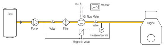
The magnetic valve opens as soon as the pressure drops below a defined level.
