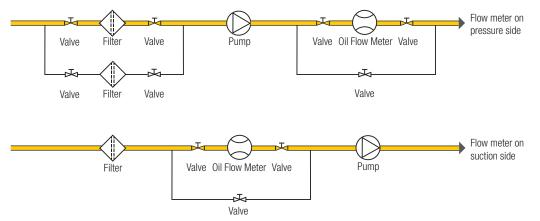
If the flow meter is installed on the suction side of the pump, the pressure drop at the max. allowed flow rate and highest possible viscosity must be taken into account. Also to be considered are installed filters.
