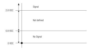
Below  $0.8\ VDC = no\ pulse\ (logic\ 0)$ Between  $0.8-2.8\ VDC$  is not defined Over  $2.8\ VDC = pulse\ (logic\ 1)$
