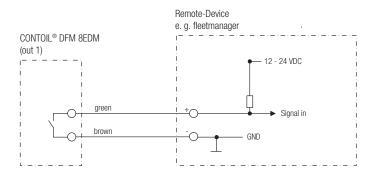
Whenever a pulse is generated, the electronic switch at the DFM 8EDM will be closed and the incoming 12-24VDC will be redirected to the external device.
