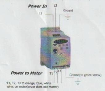
Your Extreme (6000 rpm) motor should be 230v 3 phase motor. The included GS1 controller converts the power from your region's standard voltage, listed on the controller to run the 230V 3 phase motor. So you can run your 120V or 230V single phase power into the GS1 Controller, GS1-10P5 accepts 120V single-phase power, while the GS1-20P5 accepts 230V single phase power.
