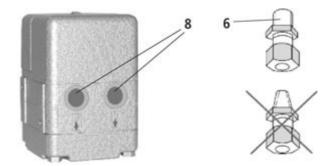
6. Remove sealing plugs [8] from the back of the oil meter and screw in screwed plugs [6] **with cylindrical threads.**
