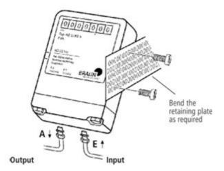
7. Attach oil meter [1] to the retaining plate [5] using the fixing screws and washers.
