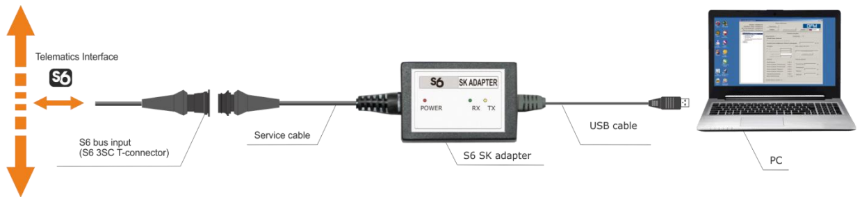
a) while using S6 SK for configuration of DFM within S6 Telematics interface
