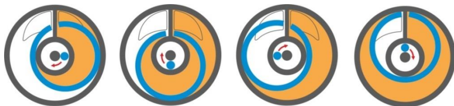
Figure 12 — DFM measuring chamber operation scheme
