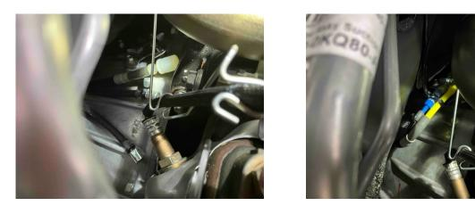
15 In the engine bay, make a final cut to length for the silencer, push the BSPP (Parallel) Pneumatic Stud Coupling on to the nylon tube, pull on the tube to make sure it is gripped in properly, screw on the Stainless Steel Socket, and finally the silencer with a spot of studlock.
