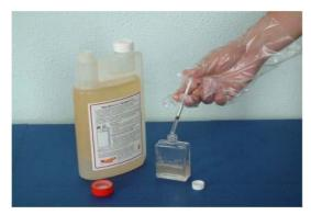
1. Break and discard the plastic seal. Remove the bottle cap and place on a clean surface with the inside face upwards. Use the syringe to add 0.25 ml fuel to the MicrobMonitor2 bottle (or 0.01 ml water using the sterile loop). Re-cap and label the bottle.
