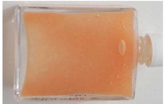
Fig. 5 MICROBMONITOR2 with colour interference due to anti-oxidant in B100
