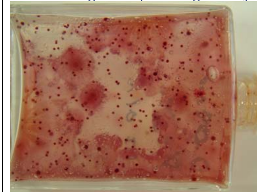
Fig. 4 MICROBMONITOR2 with normal colonies visible through the spreading colony (patch)
