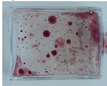
Fig. 3 MICROBMONITOR2 Tests showing development of spreading colonies over time
