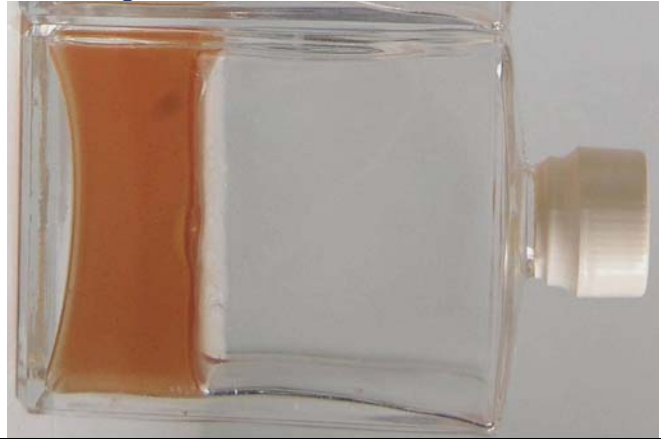
Fig. 8 MICROBMONITOR2 showing discolouration due to age (exceeded shelf life).
