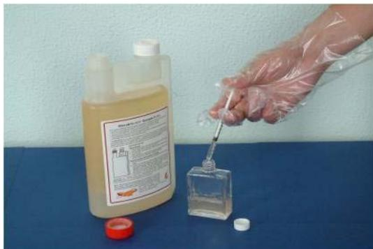
1. Break and discard the plastic seal. Remove the bottle cap and place on a clean surface with the inside face upwards. Use the syringe to add 0.25 ml fuel to the **MicrobMonitor<sup>2</sup>** bottle (or 0.01 ml water using the sterile loop). Re-cap and label the bottle.
