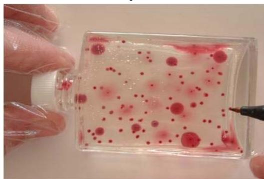
6. To examine test, hold bottle against a light background and count all of the red / purple colonies, marking them off on the bottle with a felt tip pen. Re-incubate and examine if necessary for up to 4 days (see Notes). If numbers are high an estimate can be made by comparison to the chart provided. Record all results and sample information.
