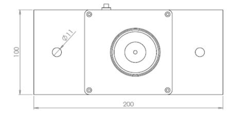
**Spring loaded centre** overcomes any residual magnetic force when the electromagnet is de-energised
