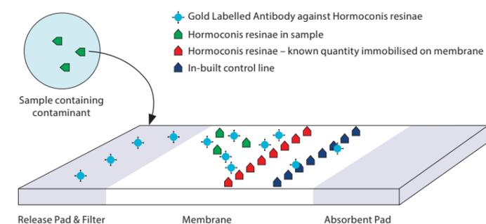
The gold-labelled antibody is immobilised in the Release Pad under the sample well. The sample containing an unknown amount of contamination is added to the sample well and this re-hydrates, allowing the reagents to flow up (wicking) the membrane towards the absorbent pad. Any large particles in the sample, which may
