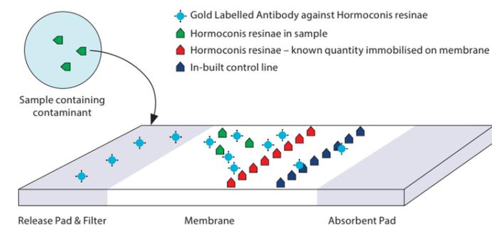
The gold-labelled antibody is immobilised in the Release Pad under the sample well. The sample containing an unknown amount of contamination is added to the sample well and this re-hydrates, allowing the reagents to flow up (wicking) the membrane towards the absorbent pad. Any large particles in the sample, which may
