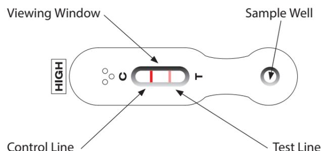
There is an in built Control in the test and for all samples run; a line should appear against the C (Control) point in the viewing window. If no line appears the test has failed and should be repeated.
