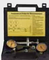
For ventilation, pressure setting and testing, vacuum and leak testing of the pump and oil line
