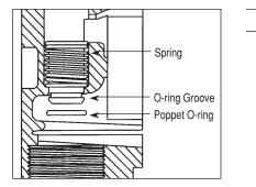
c. From inside the housing, use a small screwdriver to push the poppet and spring through the top outlet port. (Figure 11)
