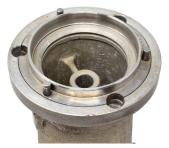
**NOSE INSERT** REPAIR MEGGITT (WHITTAKER) NOZZLE BODY REINFORCEMENT
