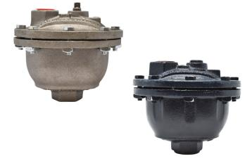
There is no question in our opinion: these are the most reliable air eliminators money can buy. Stainless steel float and mechanism, Viton A seal, 3/4" NPT in and out. (1/2" on special order), 1/16" air outlet orifice operates up to 208 psi. Air release rate at 150 psi is 6.04 cfm. Larger orifice sizes: 3 available on special order but operating pressures decrease. Structural pressure rating is 250 psi on all models. Repairable replacement parts are available.
