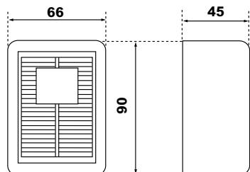
**DISPOSITIVI DI RIVELAZIONE FUGHE GAS / GAS LEAK DETECTOR DEVICES****Schema esplicativo**
