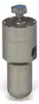
Filtro autopulente alta pressione per gasolio, olio combustibile. Attacchi 1" x 1", P.max 30 bar. High pressure self cleaning filter for oil, heavy oil. Connection 1" x 1", Pmax 30 bar.
