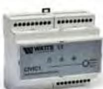
*Gas leak detection central unit for connection with one sensor Series UR13 or UR 20S with LED optical (power supply, failure, gas alarm) and acoustic interface through internal buzzer. Control output connection for gas alarm and Open Collector (OC) output connection for fault signal. Self-extinguishing plastic casing for DIN rail mounting.*
