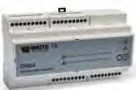
*Gas leak detection central unit for connection with four sensors Series UR13 or UR 20S with LED optical (power supply, failure, gas alarm) and acoustic interface through internal buzzer. Control output connection for gas alarm and Open Collector (OC) output connection for fault signal. Self-extinguishing plastic casing for DIN rail mounting.*
