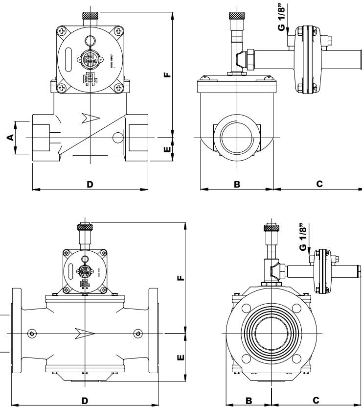
**\*) Attacco G1/8"** da collegare a valle del regolatore. - **G1/8"** connection to connect downstream the regulator.
