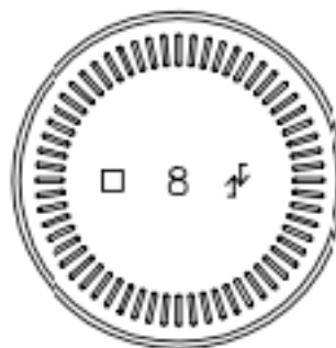
VIEW ON BASE SHOWING EMBOSSED MARKING STANDING AREA EMBOSSED WITH BAR STIPPLE
