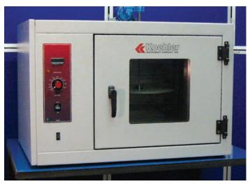
K45850 Loss on Heat / Thin Film Oven
