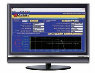
Oxidata® Software automatically calculates and displays the endpoint of RPVOT (RBOT)/TFOUT test methods.
