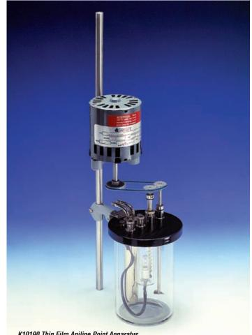
K10190 Thin Film Aniline Point Apparatus
