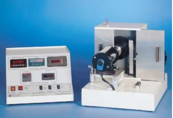
K18500 High Temperature Wheel Bearing Grease Tester
