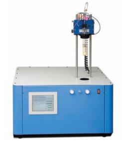
KLA-4-TS Automatic CFPP Analyzer with Integrated Touch Screen PC
