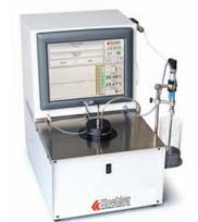
KLA-6 Automatic Filter Plugging Tendency Analyzer (FPT)
