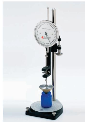
K19500 Penetrometer with K20800 Penetration Cone
