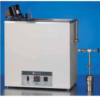
K10404 Liquid Oxidation Bath with K10500 Pressure Vessels
