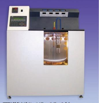
K22754-OS Digital Refrigerated Kinematic Viscosity Bath
