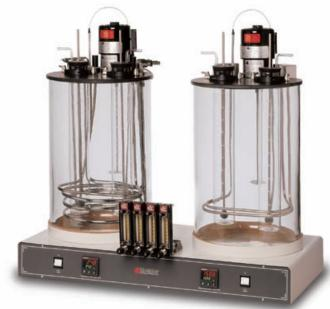
K43092 Dual-Twin Foaming Characteristics Apparatus
