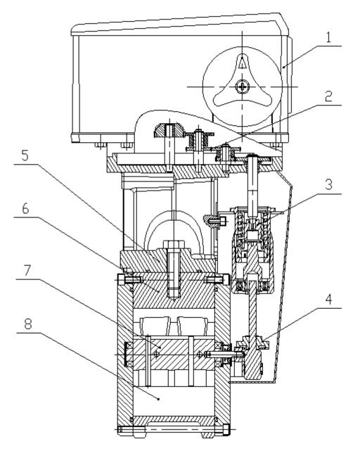
Mechanical Register 2.Gear Assy. 3. Adjuster
