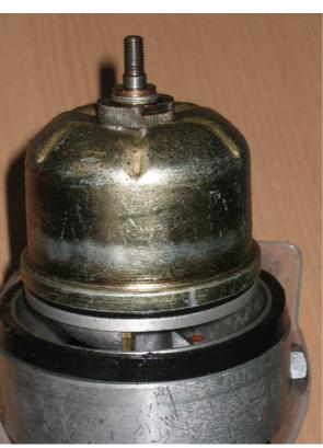
You can see the nut remains in the original position, but the Rotor Cap has lifted upwards, and the black O'ring that normally seals it against the Rotor has become visible.
