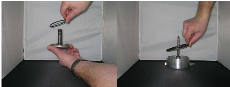
Remove Rotor O'Ring, clean & check condition
