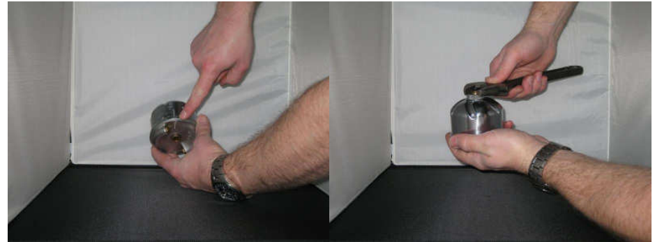
Ensure Arrow Marks match on Cover and Base
