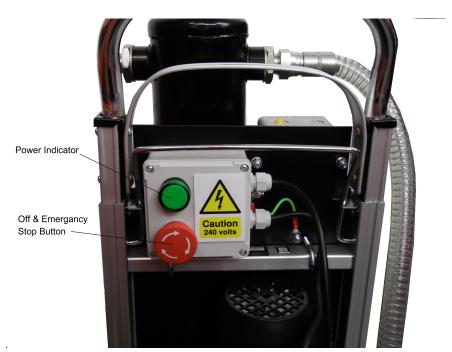
Do NOT insert or remove the power plug to start or stop the unit.
