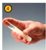
After tube fills, shake for 15 seconds. Set upright to allow powder to settle.
