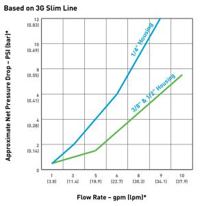
\* Pressure drop and flow rate based on housing without cartridge.
