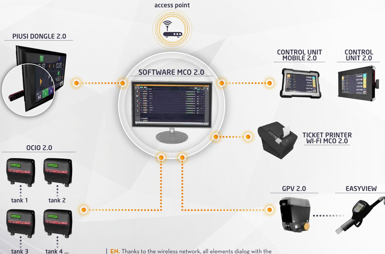
**EN.** Thanks to the wireless network, all elements dialog with the heart of the system: the MCO 2.0 software.
