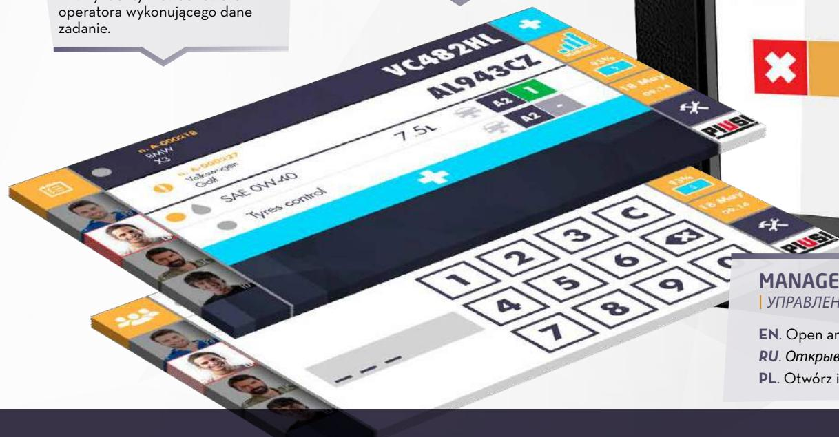
**EN** | With just a click the operator can **accept the work task**, displaying all the details and specifying, if necessary, **which fluid** will be used and the **preset quantity**. On completion, each work task is closed and recorded.
