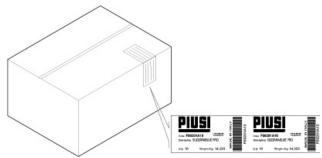
The dispensing system comes packed in a cardboard box bearing a *label* containing all the information relating to the equipment (model, weight, etc.).
