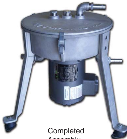
15. Wrap all male threads with Teflon Tape. Screw (1) Hose Barb into (1) 90° Elbow and (2) Plugs into Lid. Use (1) Hose Barb in place of (1) Plug if you are going to vent the Lid.
