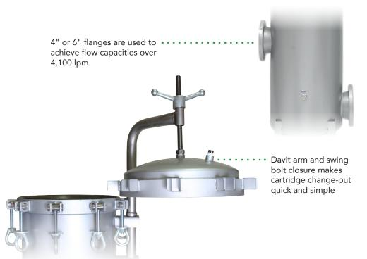
Adjustable top plates • • • • accept variable length filter cartridges
