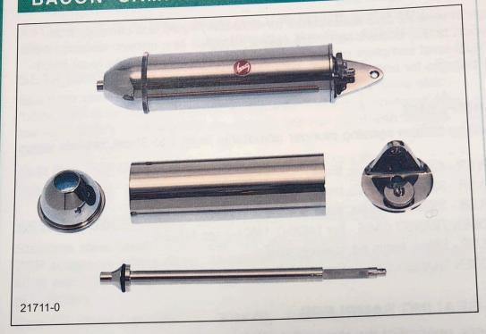
These consist of a heavy nickel-plated brass container for non-pressurised sampling with a bottom opening valve which can be opened at any depth by an actuating cord, or self-actuated when the valve or its extender rod strikes the bottom of the storage tank. Equipped with valve-stem locking device. Various lengths of rod are available to open the valve at different distances off the bottom. Approximate capacities listed.
