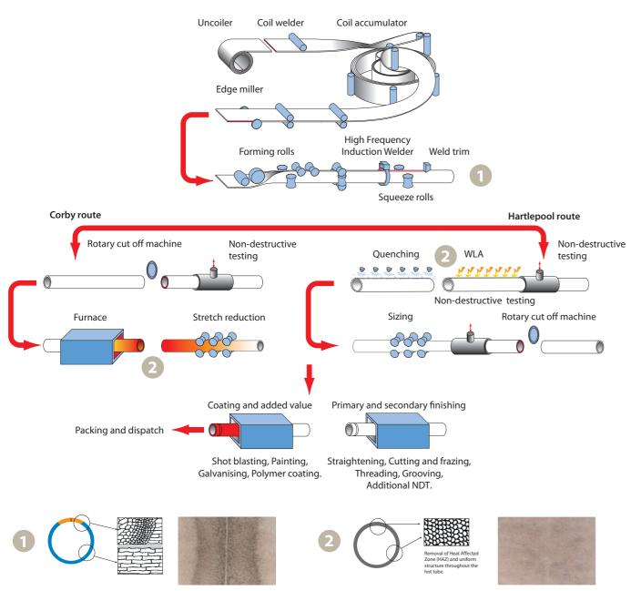
Cold-formed tube micrograph: Inconsistent structure with pockets of stress and variations in mechanical properties.
