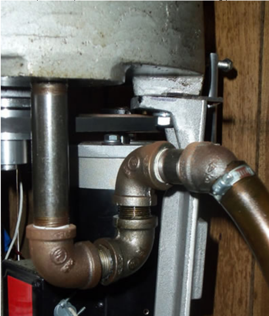
A 45 degree elbow prevents the hose from kinking.
